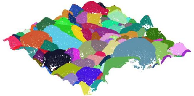
**Figure S1:** Influence of the  $k$  parameter on the initial segmentation: a)  $k=10$ , b)  $k=25$ , c)  $k=50$  and d)  $k=100$ . Each color represents the unique label of a grain obtained after the watershed initial segmentation described in section 2.1 of the main manuscript. The represented point cloud covers a square surface of  $1 \times 1 \text{ m}$ .
