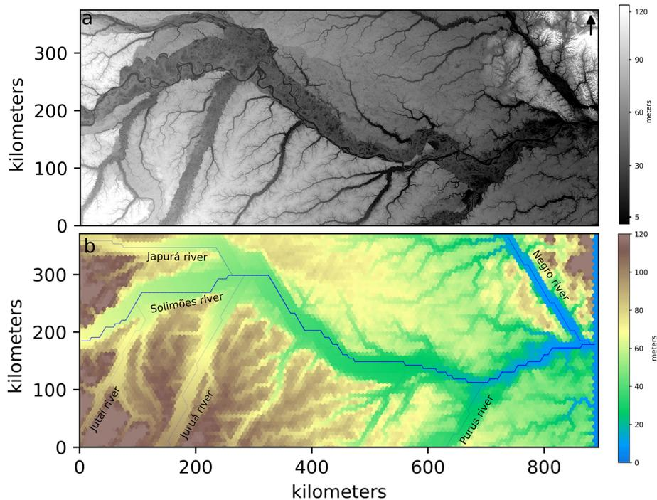
**Figure 3.** (a) Shuttle Radar Topography Mission (SRTM) digital elevation model of central Amazonia, with a resolution of 90 m at the Equator. (b) Initial topography and configuration of the numerical simulations. The blue lines represent the channels and the thickness of the line is proportional to the discharge of the corresponding stream.
