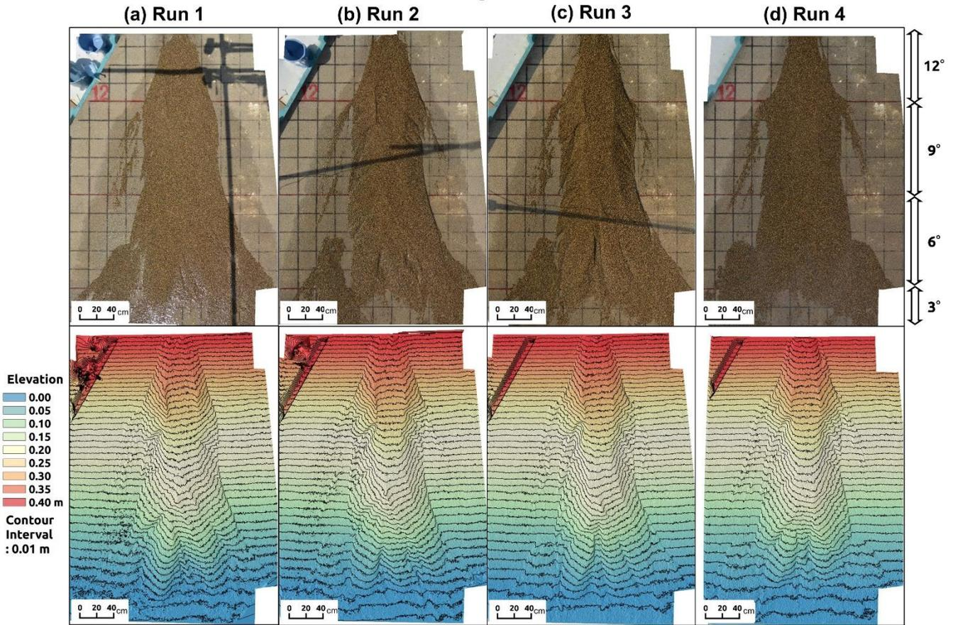
60 **Figure S6:** Final topographies of the debris-flow fans of the monogranular flows. The upper and lower panels show orthophotos and digital elevation models (DEMs), respectively. Respective sets of the upper orthophoto and lower DEM represent corresponding results of each experimental test run. The elevation of the DEMs is depicted assuming that the area with a 3° slope (i.e., the area furthest downstream from where the slope angle changed from a 6° to 3° slope) has elevation of zero.
