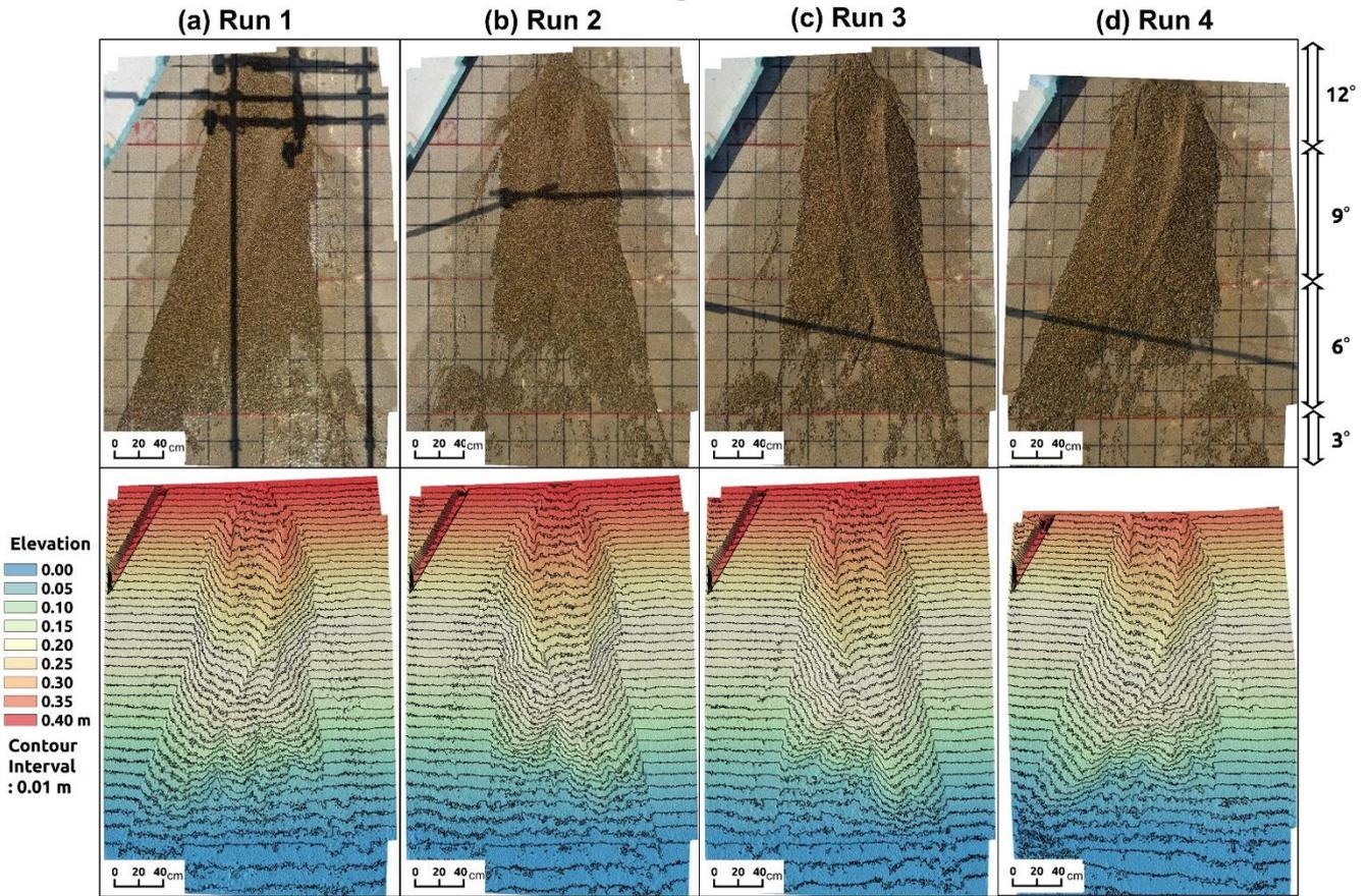
65 **Figure S7:** Final topographies of the debris-flow fans of the multigranular flows. The upper and lower panels show orthophotos and digital elevation models (DEMs), respectively. Respective sets of the upper orthophoto and lower DEM represent corresponding results of each experimental test run. The elevation of the DEMs is depicted assuming that the area with a 3° slope (i.e., the area furthest downstream from where the slope angle changed from a 6° to 3° slope) has elevation of zero.
