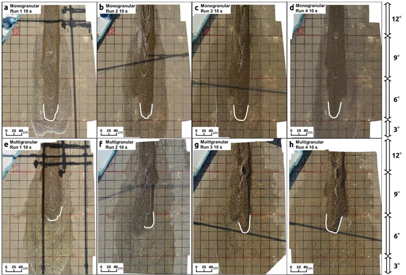
35 **Figure S3:** Orthophotos 10 s after the start of runout: (a)–(d) monogranular flows and (e)–(h) multigranular flows. The white line indicates the flow front of the solid phase.
