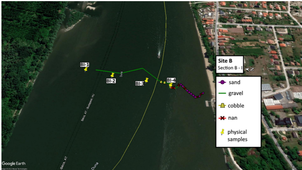
Figure E1. The path of the vessel and camera in Section B-I, Site B. The polyline is coloured based on the sediment seen during visual evaluation of the video. Yellow markers are the locations of physical bed material samplings (map created with © Google Earth Pro).
