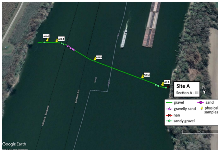
Figure D1. The path of the vessel and camera in Section A-III, Site A. The polyline is coloured based on the sediment seen during visual evaluation of the video. Yellow markers are the locations of physical bed material samplings (map created with © Google Earth Pro).
