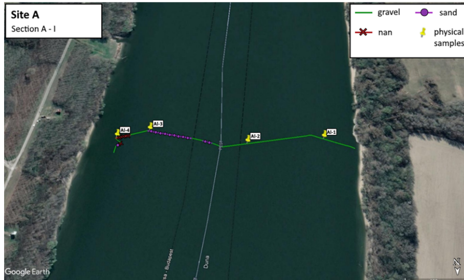
Figure C1. The path of the vessel and camera in Section A-I, Site A. The polyline is coloured based on the sediment seen during visual evaluation of the video. Yellow markers are the locations of physical bed material samplings (map created with © Google Earth Pro).
