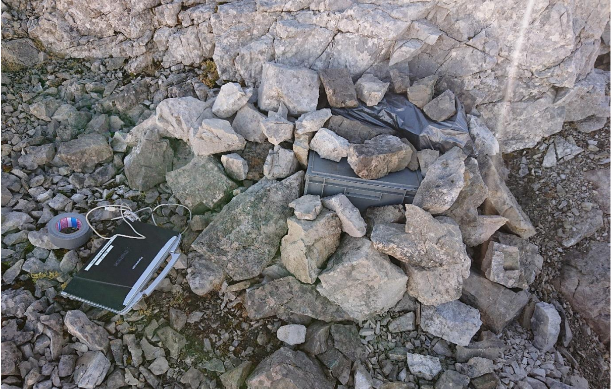
Fig. S 5: Photo of seismic station SA 22 during maintenance. During operation, the station is completely covered with rocks to protect the geophone from wind and rain.
