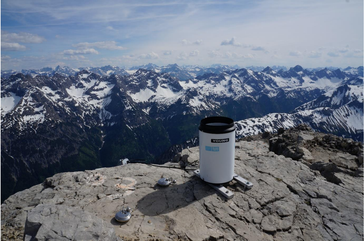
Fig. S 3: Photo of tipping bucket rain gauge on the summit of Hochvogel.
