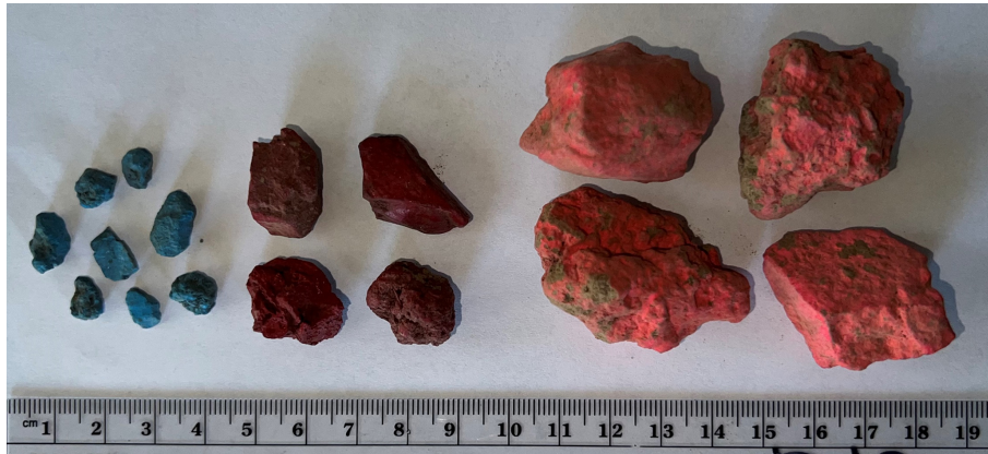
Figure 2. Examples of small (left, blue), medium (middle, red), and large (right, pink) experimental particles used in particle drop experiments in summer 2021 and spring 2022. Ruler units are in centimeters.
