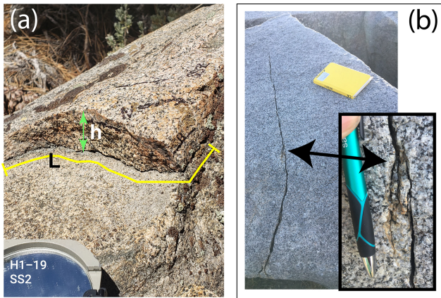
Figure 2. (a) Example of the measurement of a surface exposure length ( L ; yellow line) of a fracture meeting the criteria in Table 1. The h refers to the location where sheet height would be measured for this surface-parallel fracture. (b) Example of fractures that may appear to be a single fracture (left) but upon close examination are in fact multiple fractures intersecting and/or separated by rock (right inset). Arrow points to the location of the inset image on the main image. Labeled compass in the foreground for scale and sample location information.
