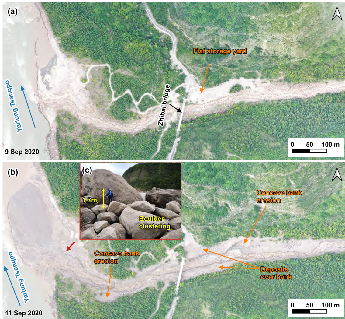
Figure 7. Comparison of pre- and post-event aerial photos on the downstream channel and alluvial fan. (a) the UAV photo on 9 September 2020; (b) the UAV photo on 11 September 2020; (c) on-site picture of the boulder clustering on 11 September 2020 (the camera angle direction is denoted by red arrow in panel b).
