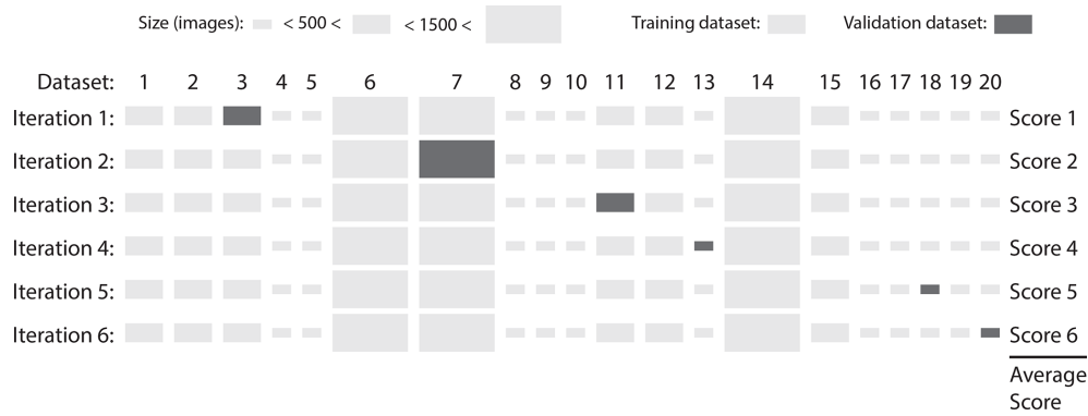
Figure 4. Cross-validation scheme for one training scenario. This figure shows the distribution between the datasets used for training and those used for validation. The y axis shows all available datasets, and the x axis shows the different training efforts. The dark-grey dataset represents the validation data, while the other 19 datasets were used to train the model. Ultimately, the six scores were averaged to produce the validation score. The size of the rectangle represents the size of the dataset.
