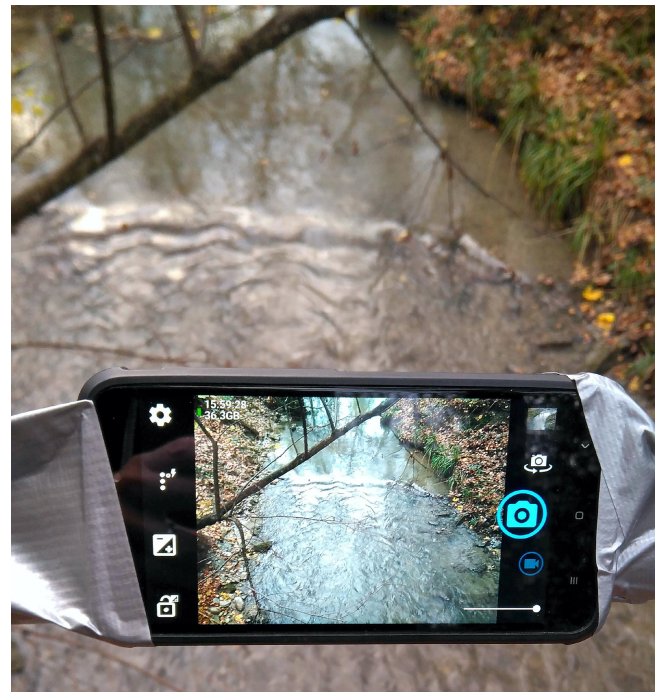
Figure B1. Example image of the data acquisition (dataset 5). A mobile phone camera was securely mounted with duct tape, providing a stable view of the river’s surface from a bridge.
