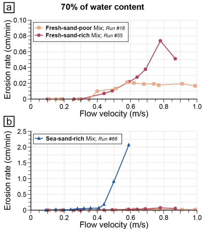
**Figure 4.** Evolution of the erosion rate for a representative run for the three mixtures, with a water content of 70 %, no vertical shaking, and increasing the flow gradually. Panels (a) and (b) display the results for the same run with the fresh sand-poor and sand-rich mixtures, while an expanded vertical scale is used in (b) to highlight the results of the run with the sea-sand-rich mixture.
