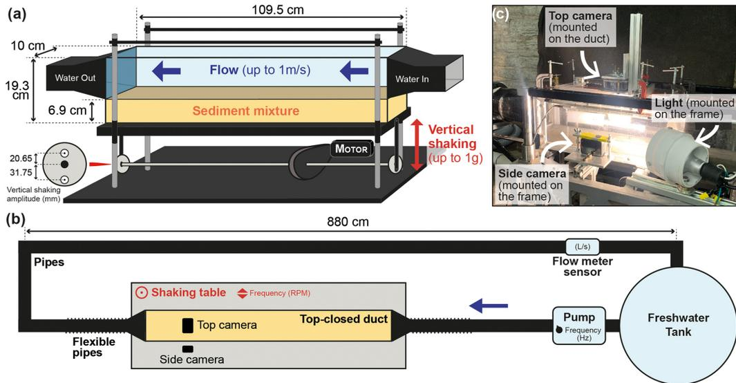
**Figure 2.** Physical experiment setup. (a) Details of the duct with sediment and water. The shaking table amplitudes are set to 20.65 or 31.75 mm for each run. (b) Top view of the system. (c) Photo of the downstream duct area targeted for data recording.
