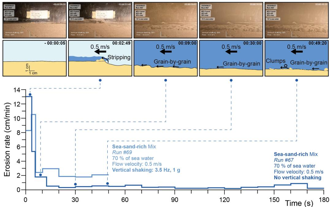
**Figure 5.** Evolution of the erosion rate of the sea-sand-rich mixture. The erosion rates are calculated over 10 s intervals but more often for the first  $\sim 10$  s of each run. The photos and their interpretative cartoons highlight different steps of run 67.
