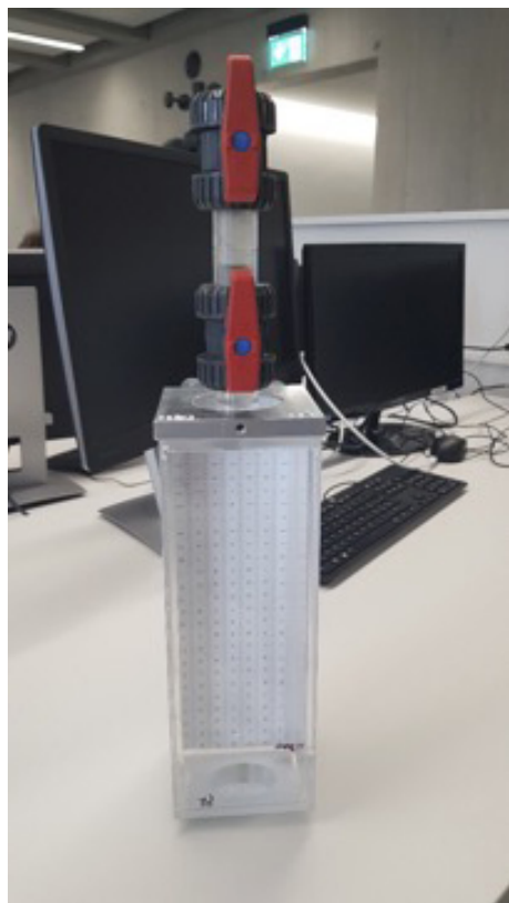
Figure 2. One of the six sedimentation chambers with the two ball valves on top. The walls are made of transparent Plexiglas and on the back wall can be seen the graph paper that is used as a visual reference for trajectory analysis of the settling particles. Image credit: Brigitte Kuhn.
