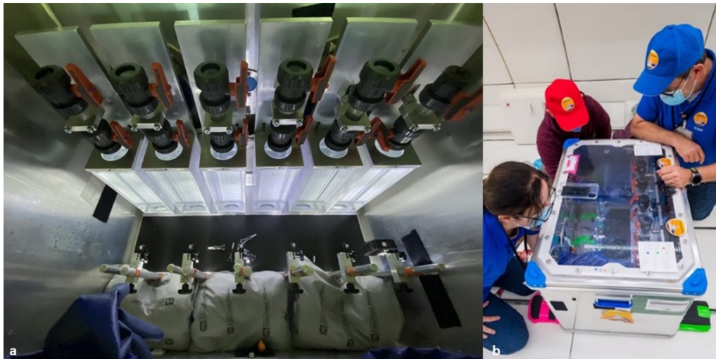
Figure 4. (a) Top view of the experimental apparatus on board the 4th Swiss Parabolic Flight Campaign held in Dübendorf Zurich (June 2020), just before the flight. The six square tubes, each filled with water and topped by two ball valves inside the aluminium containing box, are shown. In front of the settling chambers are GoPro cameras and LED lighting. Behind the GoPros, absorbent pillows, in case of liquid leakage, are visible. (b) The parabolic flight team as they manoeuvre and test the accessibility of the settling chambers using gloves inside the aircraft, the day before the parabolic flight. The team consists of four members, three of whom are visible in the figure. The blue-shirted team members, Federica Trudu on the left and Nikolaus J. Kuhn on the right, flew and performed the experiments. Image credit: Brigitte Kuhn.
