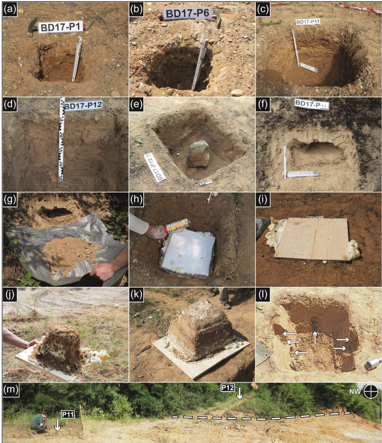
Figure S2. Pictures taken during the field tests in the gravel pit near Cologne, Germany. Different soil pits [(a) – BD17-P01; (b) – BD17-P06; (c) – BD17-P11; (d) – BD17-P12; (e) – BD17-P12.1] and a cavity [(f) – BD17-P13] were dug into gravel and loess layers within a radius of ~50 m. The excavated material was collected on a tarp (g) and weighed afterwards using a digital spring balance (luggage scale). The pits were filled with polyurethane foam and polystyrene blocks in order to obtain casts reflecting the volume of the respective pit after cooling (h-k). Small cores were taken from some sites, including BD17-P12 [(l);
