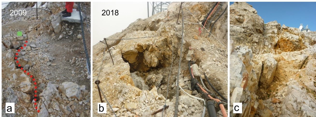
Figure S2: Growing doline at the crestline of the Zugspitze summit, at the intersection of SZ1 and SZ2 (a) in 2009 and (b) in 2018. (c) Shear zone filled with fine material.
