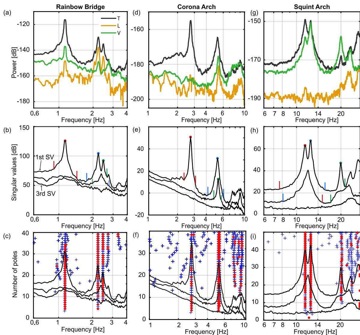
**Legend SSI plot:** + new poles   ● stable poles (frequency, damping, mode shape)
