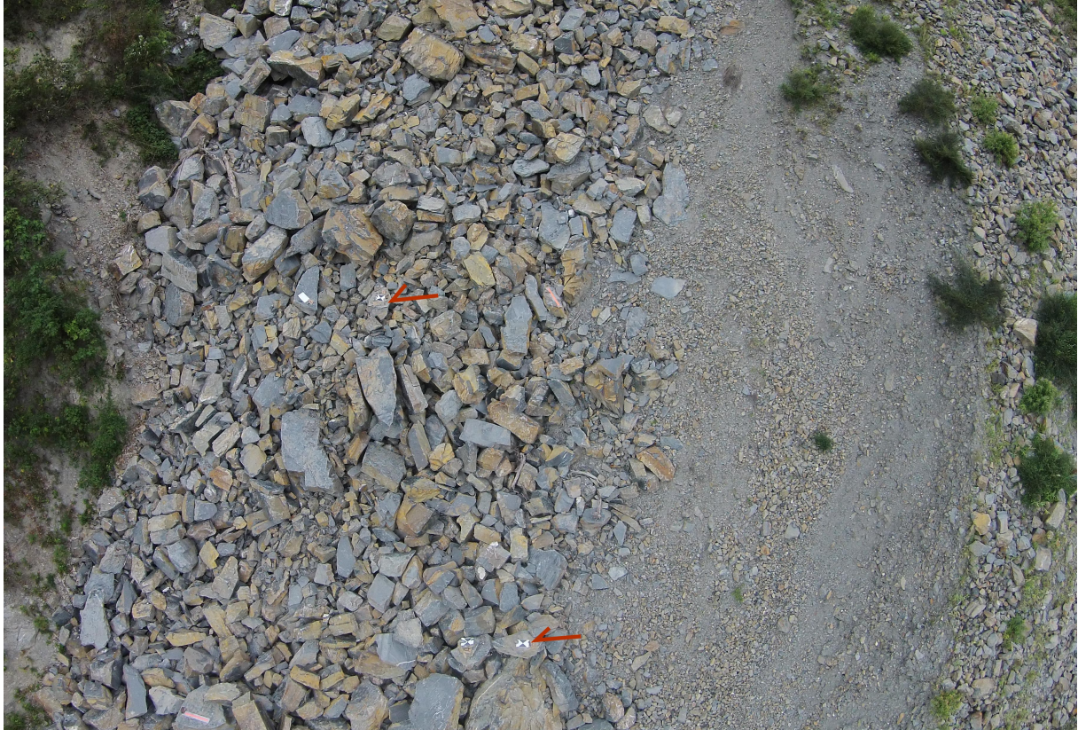
Figure S2. Drone picture above a section of the transport channel of LS-2. Note the carapace of very coarse boulders ( > 1\text{ m} , see black and white target square of 1\text{ x }1\text{ m} for scale indicated by red arrows) on the left part of the channel. On the right part the carapace is missing or eroded and finer and more variable grain sizes are visible.
