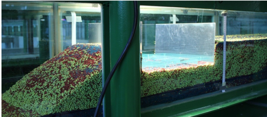
Fig. 3. Experimental set-up. Side view of the delta progradation experiment during the removal of sediment layers and sampling for sieving purposes.
