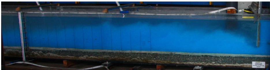
Fig. 3. Image of experiment S9. It can be seen on the right the inlet chamber, and the inlet section controlled by the sluice gate.
