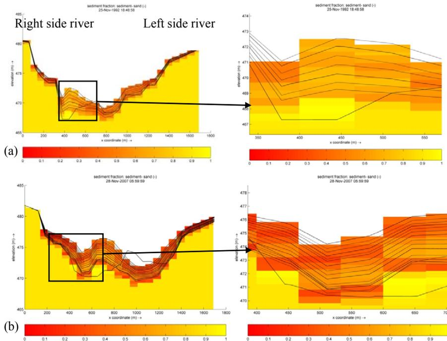
**Fig. 8.** Vertical profiles of bed composition in Area 1 seen from downstream. Left: entire cross-section. Right: zoomed areas. **(a)** period 1985–1992, **(b)** period 1992–2007. Colour bar: sand content from 0 (red) to 100 % (yellow).
