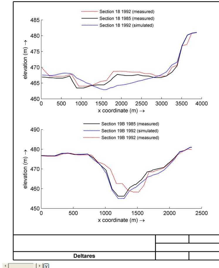
**Fig. 5.** Cross-sections 18 and 19B seen from downstream. Measured 1985 and 1992 bed elevations and simulated 1992 bed elevation. Cross-section 18 and 19B are located 10.8 km and 15.4 km upstream of the dam, respectively.
