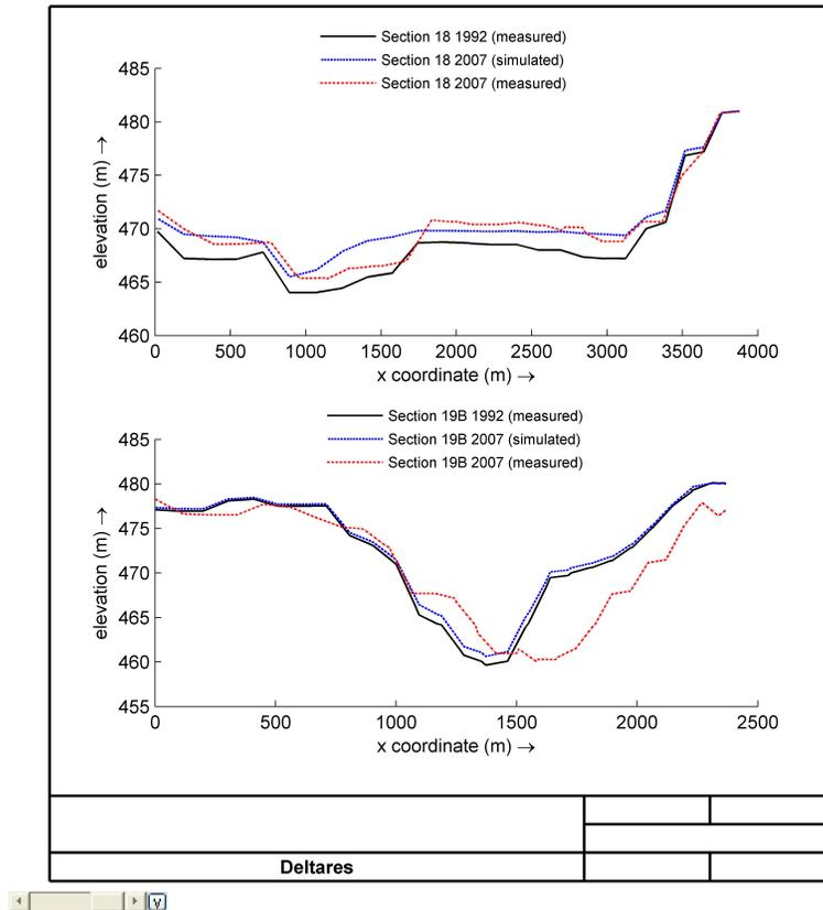
**Fig. 6.** Cross-sections 18 and 19B seen from downstream. Measured 1992 and 2007 bed elevations and simulated 2007 bed elevation. Cross-section 18 and 19B are located 10.8 km and 15.4 km upstream of the dam, respectively.
