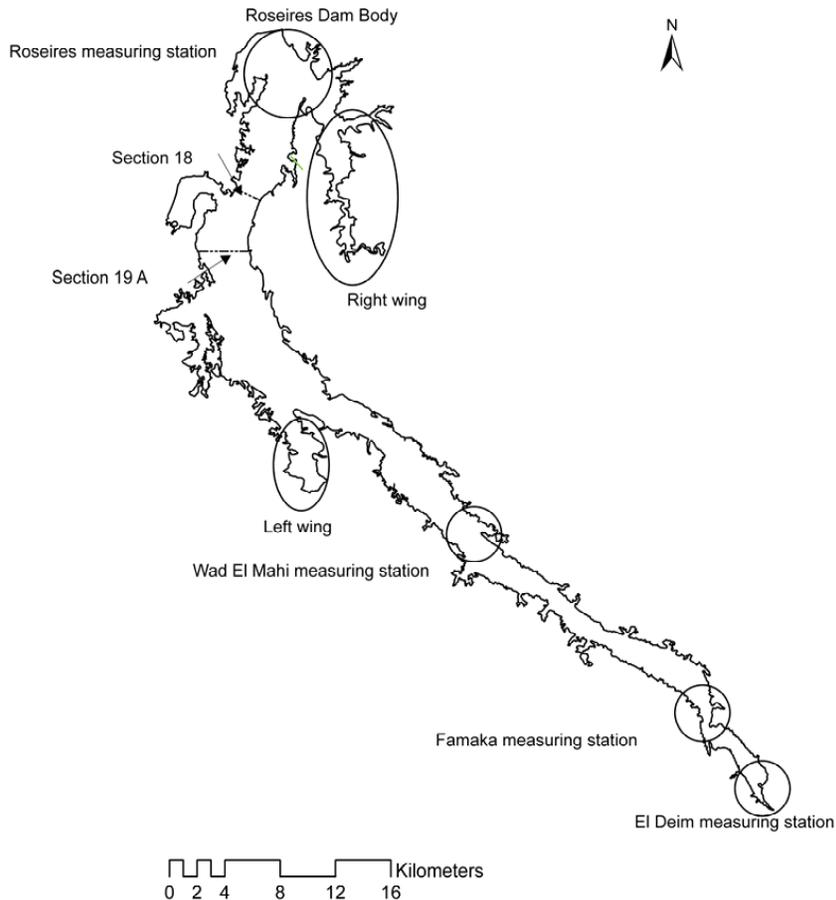
**Fig. 2.** Measurement stations and the areas (circled) that are not covered by the surveys of 1985 and 1992. The thick black line represents the contour of the reservoir at an elevation of 481 m.a.s.l. (Irrigation Datum).
