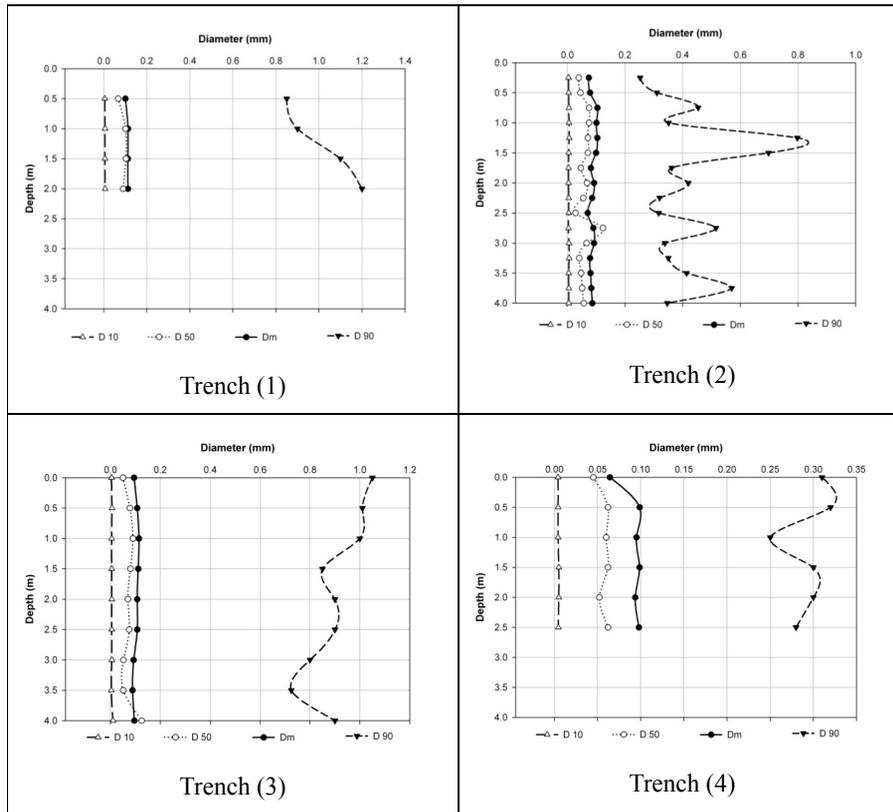
**Fig. 9.** Soil stratification at the four trenches.
