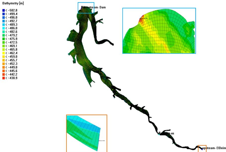
**Fig. 3.** Upstream and downstream boundaries, computational grid and bed elevations in 2009, in m.a.s.l. (Irrigation Datum).
