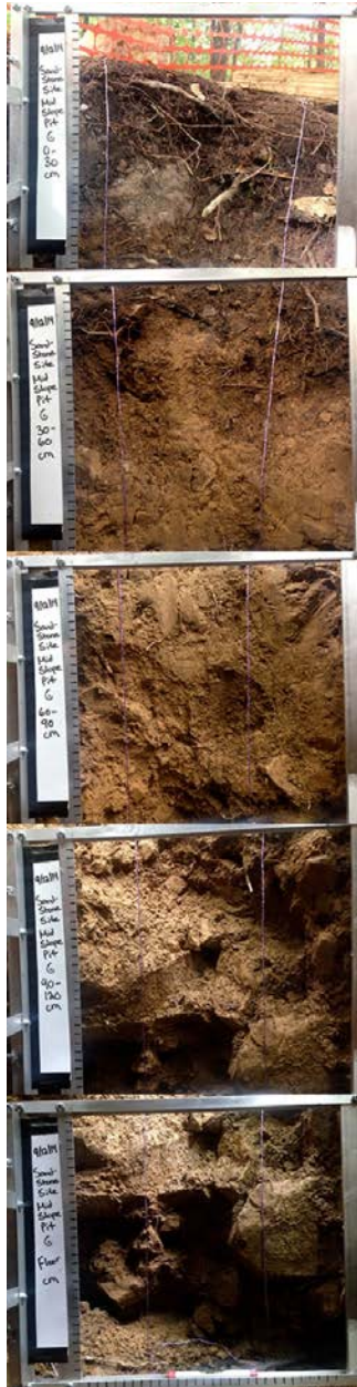
Figure S3. Photographic montage of depth intervals of the TMMS pit in the Garner Run subcatchment. The five images from top to bottom show the following depth intervals: 0 to 30 cm, 30 to 60 cm, 60 to 90 cm, 90 to 120 cm, and 120 cm to bottom. Soil description is summarized in Table S2. Photos show decreasing root density and increasing rock size with depth. The uppermost layer of large rocks can also be seen.
