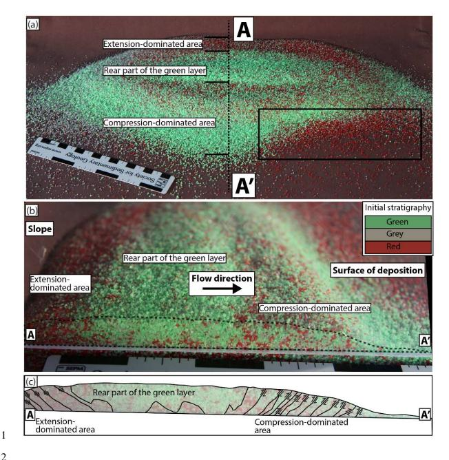
Figure 11: (a) analogue result of the experiment carried with 3 colored sands (Figure 10); (b) cross-section AA' through the center of the analogue deposit; (c) interpretation of the cross-section AA'.
