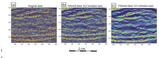
3 Figure 5: Application of the median filter to remove noises. (a) Original data; (b) Filtered
