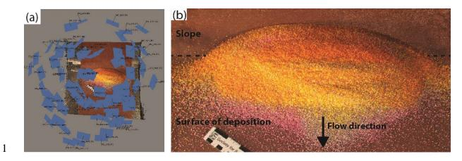
3 Figure 4: (a) View of the different position of the camera to take pictures for structure-from-
