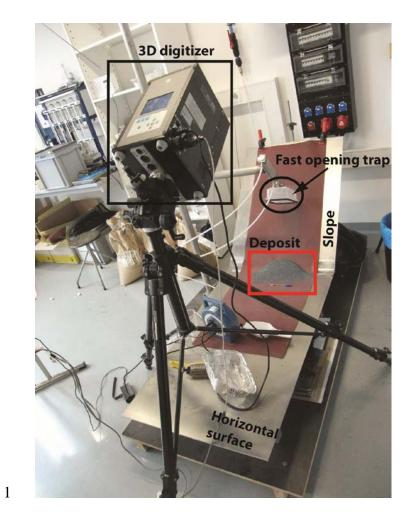
3 Figure 2. Laboratory setup.
