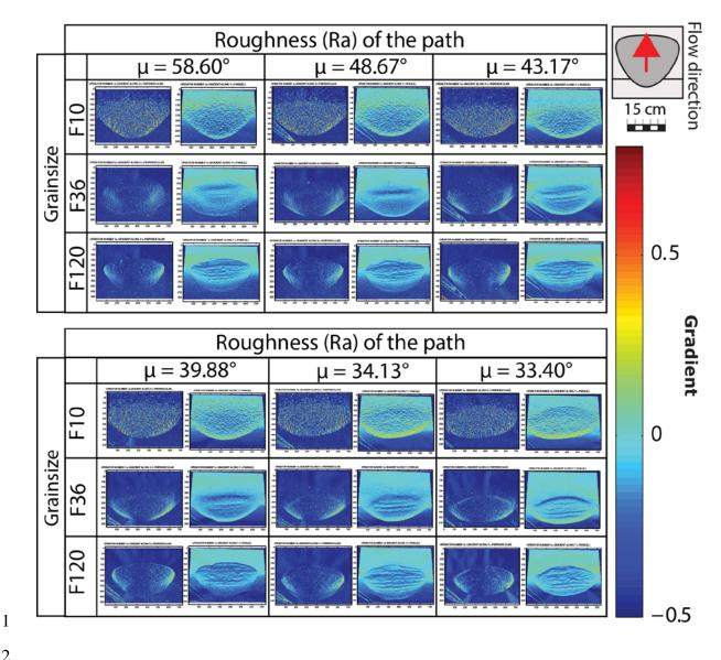
Figure 7: Results of the gradient along X and Y applied to all experiments carried for this research. The best results are obtained with the gradient along Y. The influence of the grainsize and the substratum on the shape of the deposit is clearly observable.
