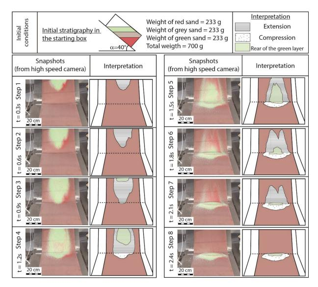
Figure 10: Time laps of an analogue granular flow (0.3 second between each picture). Three colored sand were used during this experiment (red, grey, green). On the left column are the snapshots of the experiment and the right column the interpretation of the flowing mass.
