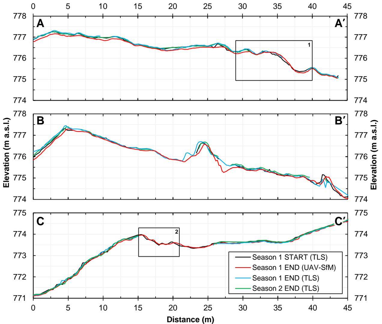
**Figure 4.** Moraine surface elevation profiles, extracted from gridded ( $0.2 \text{ m}^2$ ) digital elevation models of TLS- and SfM-derived topographic datasets. Profile locations are shown in Fig. 4. Profiles A and B bisect the main central moraine crest, whilst profile C is located on moraine deposits at the back of the embayment. Inset numbered boxes in profiles A and C show areas referred to in the text.
