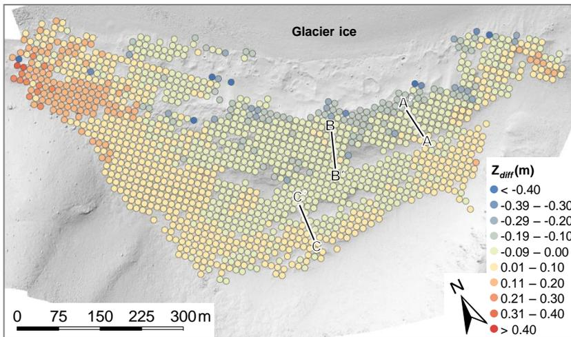
**Figure 3.** Results of vertical ( $Z_{diff}$ ; m) differencing of the UAV-SfM and TLS datasets acquired at the end of season 1, represented as the average difference within 10 m<sup>2</sup> grid cells. 83% of the UAV-SfM data were found to be within  $\pm 0.1$  m of the equivalent TLS data. Profiles A-C are displayed in Fig. 4.
