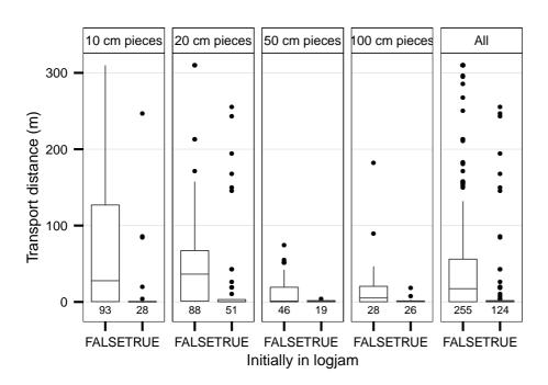
**Figure 6.** Transport distances of the tracer logs that were situated within or outside a log jam before the discharge event. The data is presented for four classes of pieces of different length. The number below the plot gives the number of data points used in the analysis. The differences in median transport distances between pieces inside and outside log jams in the 10 and 20 cm classes, as well as for all pieces combined, are highly significant.
