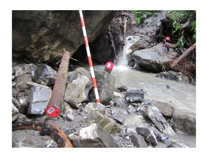
Figure 2. Tracer log with length 100 cm lying loose on the Erlenbach channel surface in the foreground. Other tracer logs are visible in the background.
