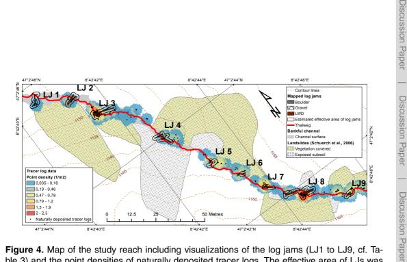
**Figure 4.** Map of the study reach including visualizations of the log jams (LJ1 to LJ9, cf. Table 3) and the point densities of naturally deposited tracer logs. The effective area of LJs was estimated by adding a buffer of 1 m around the mapped LJ perimeter to account for survey inaccuracy.
