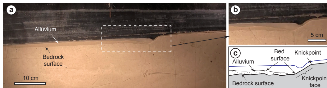
Figure 3. Illustration of a knickpoint observed along the flume during experiment #10. (a) Over-all view of the profile and (b) (c) details of the knickpoint. Note the white color of the water due to suspended sediments.
