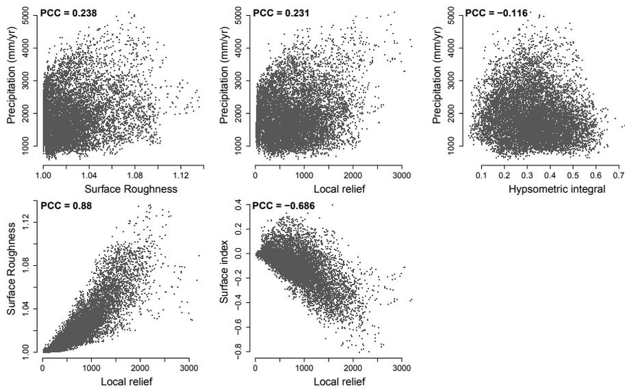
**Figure 9.** Comparison between precipitation(derived from TRMM data) and morphometric indices within the Sierra Madre de Chiapas. Points represents pixel values extracted from the precipitation (Fig. 5b) and morphometric maps (Fig. 7 and 8). The linear correlation between the variables was estimated using the Pearson correlation coefficient (PCC).
