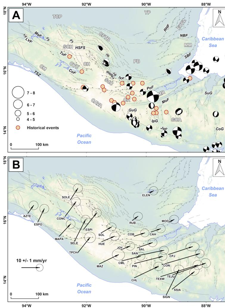
**Figure 3.** Superficial (depth <40 km) seismicity in northern Central America (A) and GPS velocities with respect to the fixed North American plate (B). Focal mechanisms from Guzmán-Speziale et al. (1989); Guzmán-Speziale (2010) (in greys) and Global CMT Catalog (in black, <http://www.globalcmt.org>). Historical earthquakes (red circles) from White (1984); Singh et al. (1984) and Guzmán-Speziale (2010). GPS velocities are from Franco et al. (2012). See Fig. 2 for abbreviations.
