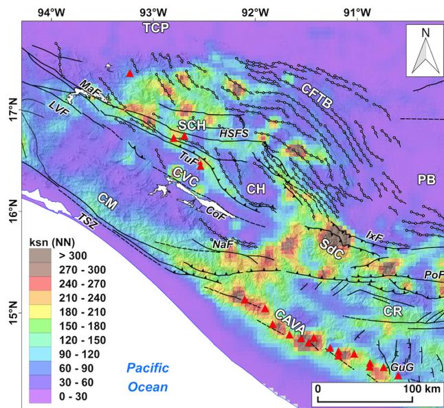
**Figure 15.** Interpolated map of steepness index ( $k_{sn}$ ) for the Sierra Madre de Chiapas and the northern segment of the Central America volcanic arc. Values were extracted from river longitudinal profiles using 5 km long segments and interpolated using a natural neighbor (NN) method. See Fig. 2 for abbreviations.
