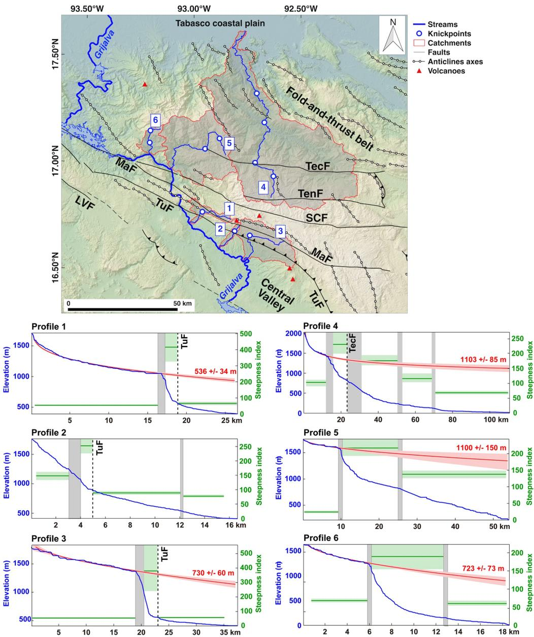
**Figure 14.** Longitudinal profiles for the Sierra de Chiapas. Channels and profiles were extracted from the modeled drainage network. See Fig. 12 for plot description. Abbreviations: LVF – La Venta fault, MaF – Malpasos Fault, SCF – San Cristobal fault, TecF – Tectapan fault, TenF – Tenejapa fault, TuF – Tuxtla fault.
