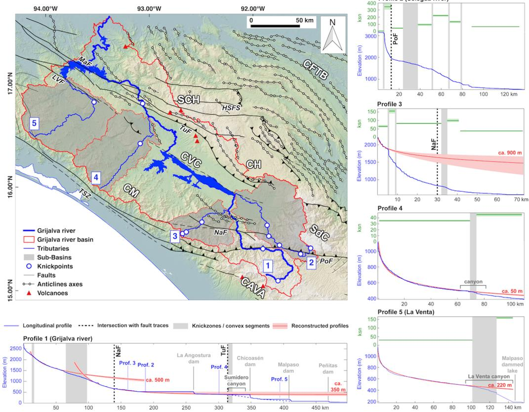
**Figure 13.** Longitudinal profiles for the Grijalva river and the tributaries from the Sierra de los Cuchumatanes and Chiapas Massif. Profiles were extracted from the modeled drainage network. See Fig. 2 for faults abbreviations and Fig. 12 for plot description.
