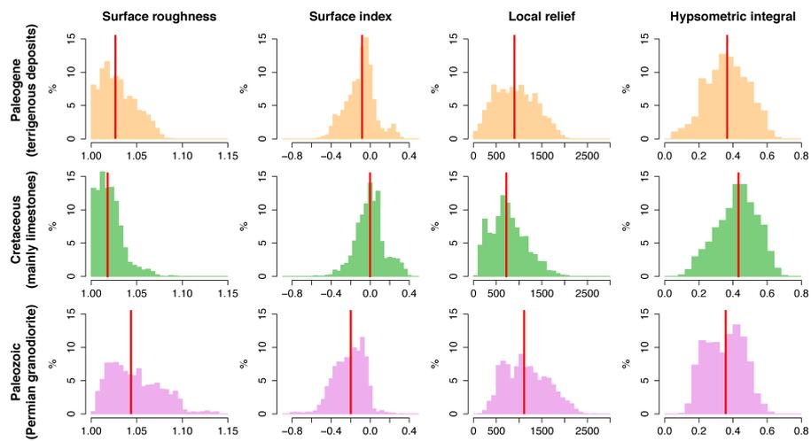
**Figure 10.** Distribution of morphometric indices for the main lithological groups of the Sierra Madre de Chiapas. Histograms are based on three sets of 5000 pixel values extracted from the morphometric maps (Fig. 7 and 8). Red line represents the median.
