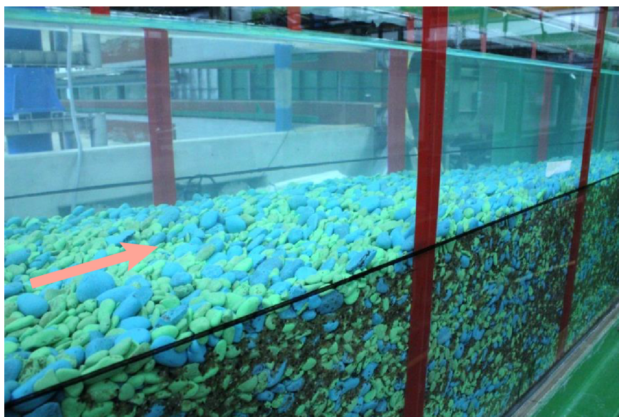
Figure 6. Imbrication of the bed surface at the end of experiment T1. Flow is from left to right.
