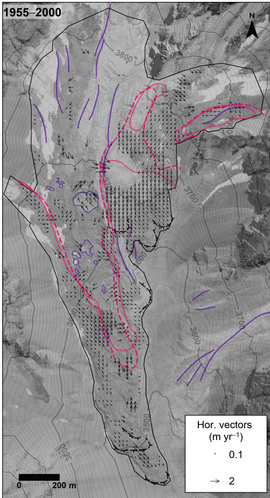
2 Figure 9. Horizontal displacements at the surface of Navarro between 1955 and 2000. The boundary 3 between debris-covered and rock glacier morphology is depicted with a dotted red line in 1955 and with 4 a dashed red line in 2014. Note that moraine crests and thermokarst depressions in 2000 are indicated. 5 The background of the map is the 2000 orthophoto.
