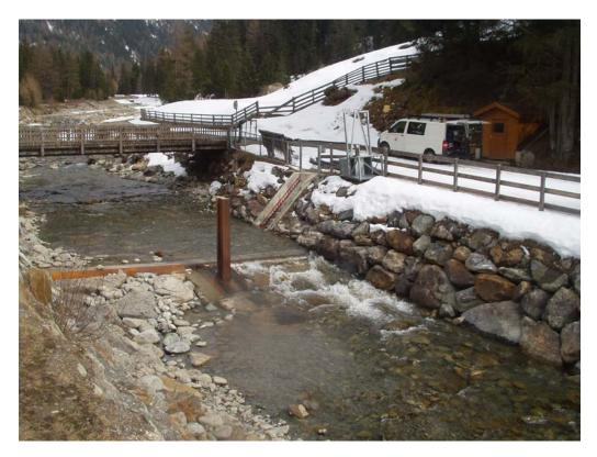
**Figure S2.** Geophone measuring cross-section at the Fischbach in March 2013, view looking upstream. Note that only about half the width of the sill with the steel plate is submerged under water. Base-flow during this period is approximately  $1 \text{ m}^3 \text{ s}^{-1}$ . (Photo Hydrographic Service of Tyrol.)
