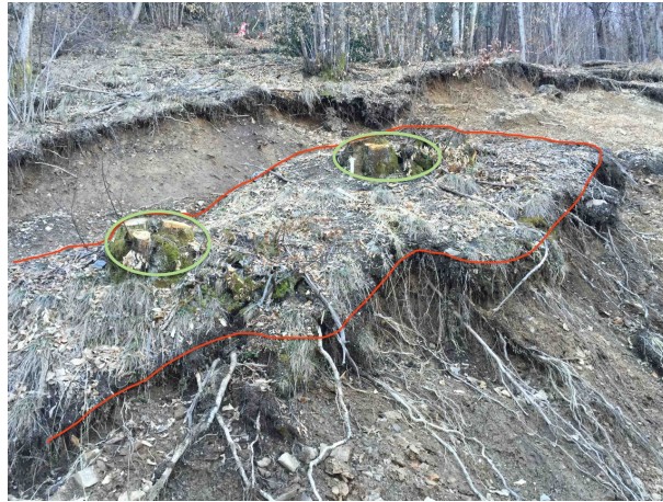
Figure 12. Example of a weak zone in a forested area showing isolated tree stumps with root system that behaved as a stiff island during the opening of a gap in a weak zone in between root systems of adjacent trees.
