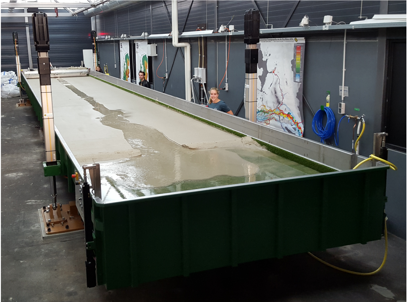
Figure 2. The Metronome tidal facility. Note PhD candidates for scale. The flume floor below the sand is covered in artificial grass (see text). Note the vertically mounted actuators that drive the flow. This pilot experiment started as a 0.2 m by 0.03 m straight initial channel and ran for about 12 hours with a slope amplitude of 0.005 m/m and a period of 30 s and 100 L/h river inflow.
