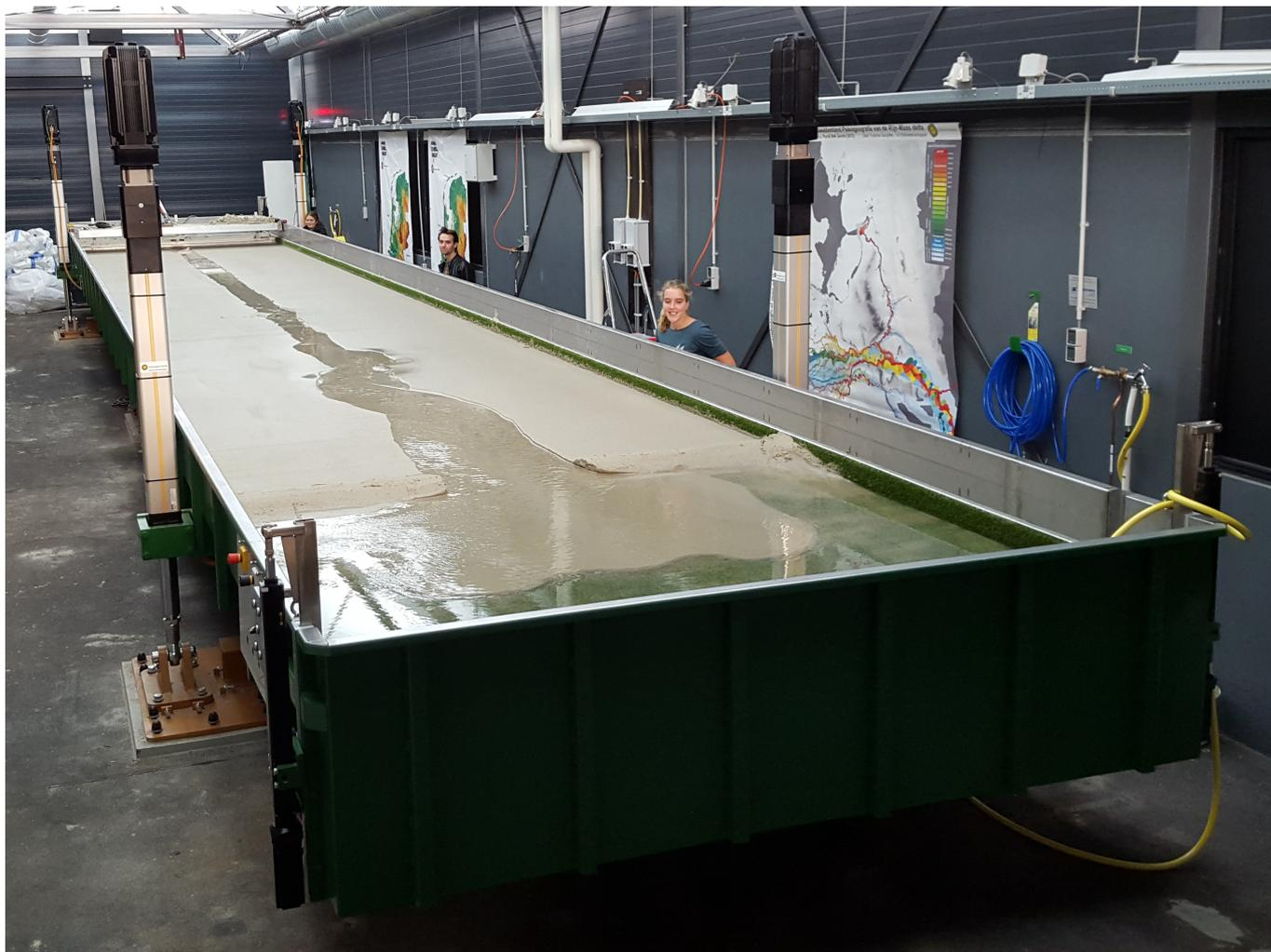
**Figure 2.** The Metronome tidal facility. Note PhD candidates for scale. The flume floor below the sand is covered in artificial grass (see text). Note the vertically mounted actuators that drive the flow. This pilot experiment started as a 0.2 m by 0.03 m straight initial channel and ran for about 12 hours with a slope amplitude of 0.005 m/m and a period of 30 s and 100 L/hr river inflow.
