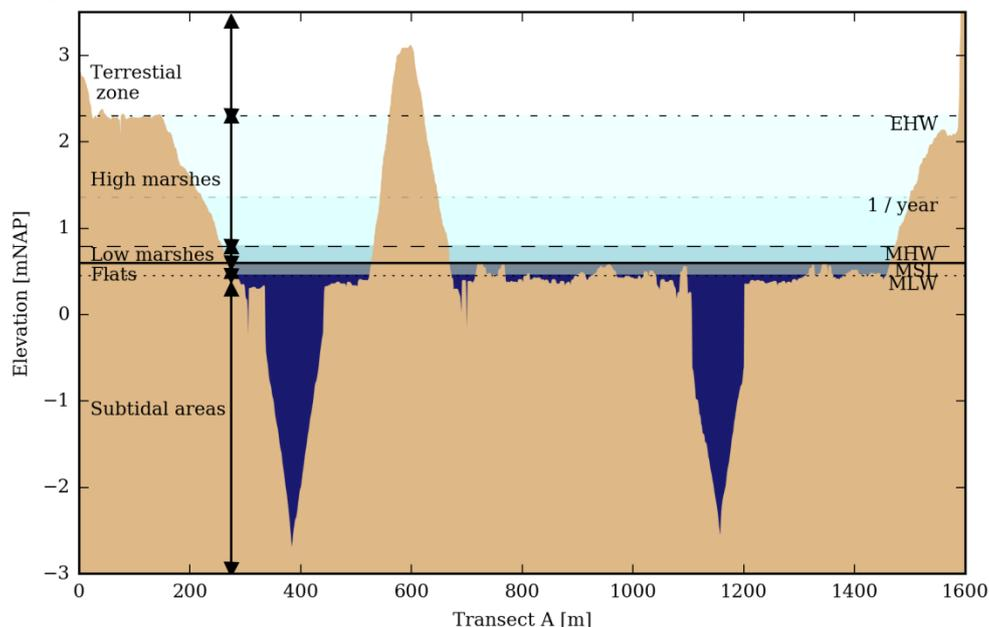
Figure 2. Elevation of Transect A (see Figure 1) with respect to the Dutch Ordnance Datum (m NAP) with subdivision of the area into subtidal areas, flats, low and high marshes, and terrestrial zone relative to mean low water (MLW), mean sea level (MSL), mean high water (MHW), the maximum observed water level (EHW) and the water level for a peak discharge or storm with return period of 1 year, which were used to divide the study area in.
