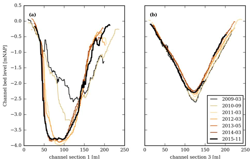
*Figure 4. Bed level of channel section 1 (a) and 3 (b) for all monitoring campaigns. (see Figure 1 for the locations of the cross sections)*
