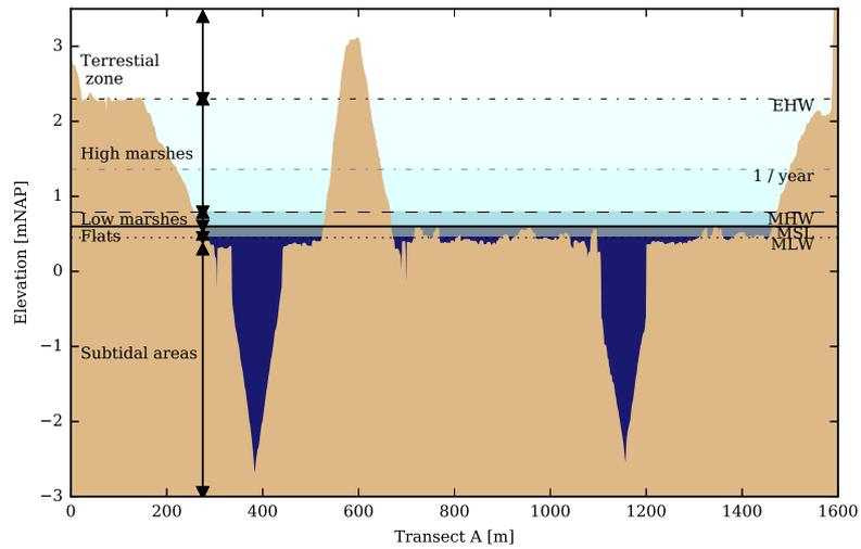
**Figure 2.** Elevation of Transect A (see Fig. 1) with respect to the Dutch Ordnance Datum (m NAP) with subdivision of the area into subtidal areas, flats, low and high marshes, and terrestrial zone relative to mean low water (MLW), mean sea level (MSL), mean high water (MHW), the maximum observed water level (EHW) and the water level for a peak discharge or storm with return period of 1 year, which were used to divide the study area in.
