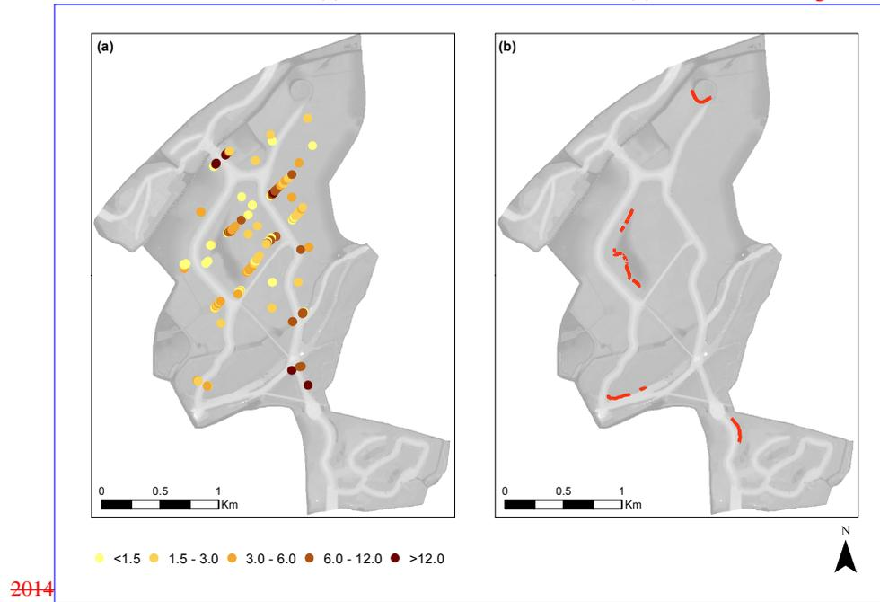
**Figure 6.** The total sedimentation [cm] in the subtidal and intertidal area (a) and the location of the cutbanks (b) as measured during field campaigns of 2014
