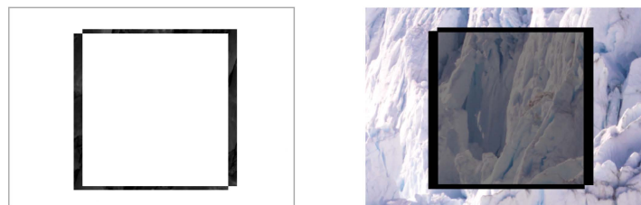
5 Figure 7: Least Squares matching with shadow pixel exclusion. The figure shows a synthetically generated image pair, which simulates a glacier motion superimposed by shadow movement, for which reference values are known (top). A method which iteratively detects and excludes shadow motion pixels from the matching is applied to this image pair (below). For each iteration step, the calculated translation parameters (left), the difference image between patch and transformed search patch (center), as well as the resulting exclusion pixels for the next iteration, which are superimposed as black pixels on the patch (right), are shown.
