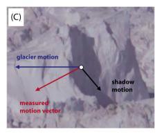
Figure 6: Influence of moving shadows in image sequences. The figure shows corresponding image sections from two sequence images recorded at a time interval of 30 min (A). In the same image pair those pixels were marked black, which are influenced by shadow motion (B). These pixels falsify the result of the feature tracking because the tracked glacier movement is overlaid by the shadow movement (C).
