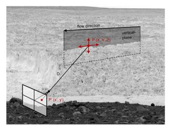
Figure 14: Transformation into object space.
