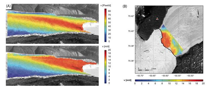
Figure 11: Result of scaling (A) and geo-referencing (B) at Støre Qarajaq glacier. The figure shows the color-coded superposition of velocity values derived from measured trajectories. They are shown as unscaled values in image space (A, top) and scaled values transferred into object space (A, bottom), as well as geo-referenced values that can be overlaid on satellite images (B).
