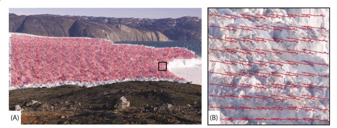
Figure 5: Raster of measurement points on the glacier surface (A) and resulting trajectories obtained from feature tracking (B). The figure shows the grid of the measuring points (red dots) as a superposition of a sequence image (A). For the black-marked area, the corresponding image section is shown on the right. It is superimposed by the measured trajectories (red lines) for a 24 h image sequence (acquisition interval 20 min) (B).
