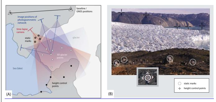
Figure 3: Combined scheme for the setup of a time-lapse camera and its corresponding geo-referencing measurement setup (A), measurement image of time lapse camera (B)
