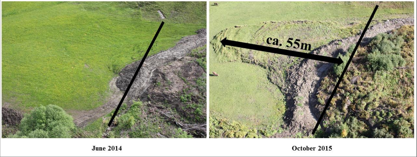
Figure 9: Aerial images illustrating the advance of the frontal lobe of the earthflow between June 2014 and October 2015.
