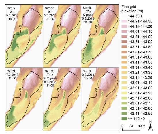
Figure 8. The bed elevations of simulation 9 (with increased transverse slope) during moderate discharge event. The key time steps are presented (cf. Figure 7).
