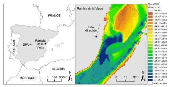
Figure 1: The study site of the Rambla de la Viuda, Eastern Spain. The elevation on March 2012 is derived mainly from mobile laser scanning data, but the edges are from the 2009 national digital elevation model. The analyzed area was defined, based on the data coverage of March 2013.
