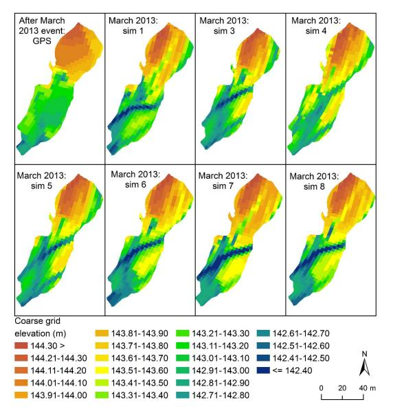
Figure 4: The bed elevations after the first March 2013 flow event (see simulation parameters from Table 4). The comparisons of the channel-bed elevations of the "analyzed area" (see Figure 1). The coarse grid cell sizes were applied in these simulations.
