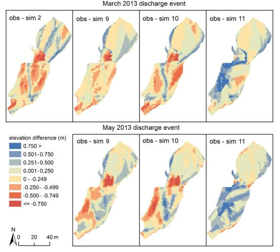
Figure 6: The comparison between the observed and simulated elevations after the March 2013 and May 2013 discharge events. The negative values (red) mean that the simulated elevations were higher in those locations. The fine grid cell sizes were applied in these simulations.
