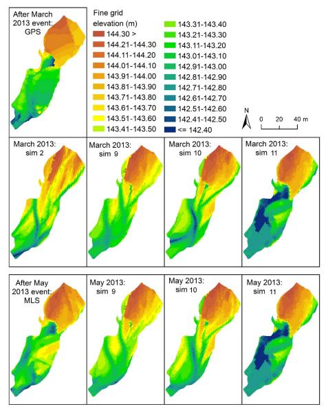
Figure 5: The bed elevations after the March and May 2013 flow events: The fine grid cell sizes were applied (see simulation parameters from Table 4). The comparisons were made against the bathymetries made, based on March 2013 GPS survey and June 2013 laser scanning data of the "analyzed area" of Figure 1.
