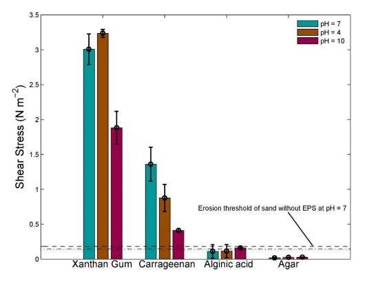
5 Figure 8. The erosion thresholds as a function of pH for four synthetic EPS as measured with the CSM erosion device. The horizontal lines correspond to the erosion thresholds of sand without EPS for water with a pH of 7 (dashed), a pH of 4 (dotted), and a pH of 10 (dash-dotted). Error bars are standard deviation from n =3 repeat measurements.
