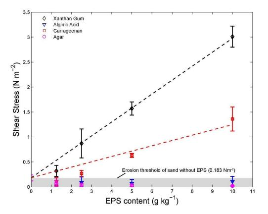
Figure 4. The erosion thresholds of 110 micron sandy substrate with different contents for four synthetic EPS as measured with the CSM erosion device. Best fit curves were fitted using linear models for Xanthan Gum (Shear stress threshold = 0.28 EPS content + 0.18) and Carrageenan (Shear stress threshold = 0.11 EPS content + 0.18). Error bars are standard deviation from n =5 repeat measurements.
