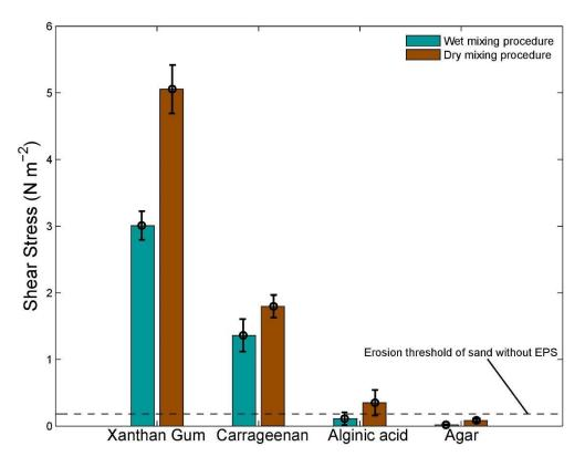
Figure 5. The erosion thresholds as a function of the preparation procedure for four surrogates as measured with the CSM erosion device. Wet mixing involves dissolving the synthetic EPS powder in water and stir, then add sediment and mix. Dry mixing involves the addition of synthetic EPS powder to sediment and mix, then add water and stir. Error bars are standard deviation from n = 5 repeat measurements.
