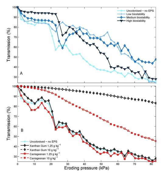
Figure 10. CSM erosion profiles for sediment with different degrees of biostability due to natural biofilm colonisation (A) and due 5 to different Xanthan Gum and Carrageenan synthetic EPS contents (B).
