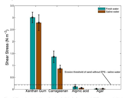
Figure 7. The erosion thresholds as a function of salinity for four synthetic EPS as measured with the CSM erosion device. Tap water
