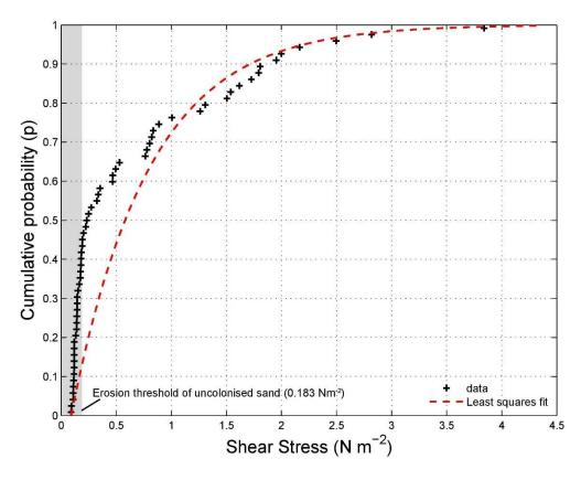
Figure 2. Shear stress measurements made with CSM erosion device during natural biofilm growth experiment. The measurements (n = 61) are best described by a least squares exponential fit with a mean parameter  $\mu$  of 0.71.
