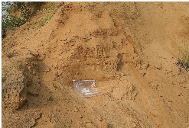
Figure A14. LH - Cross-bedded sand exposure (4 m high). Sample taken 2.2 m from top of exposure. Corresponds to OSL sample from unit dated at 23,500 \pm 1,500 years by Verma (2016).
