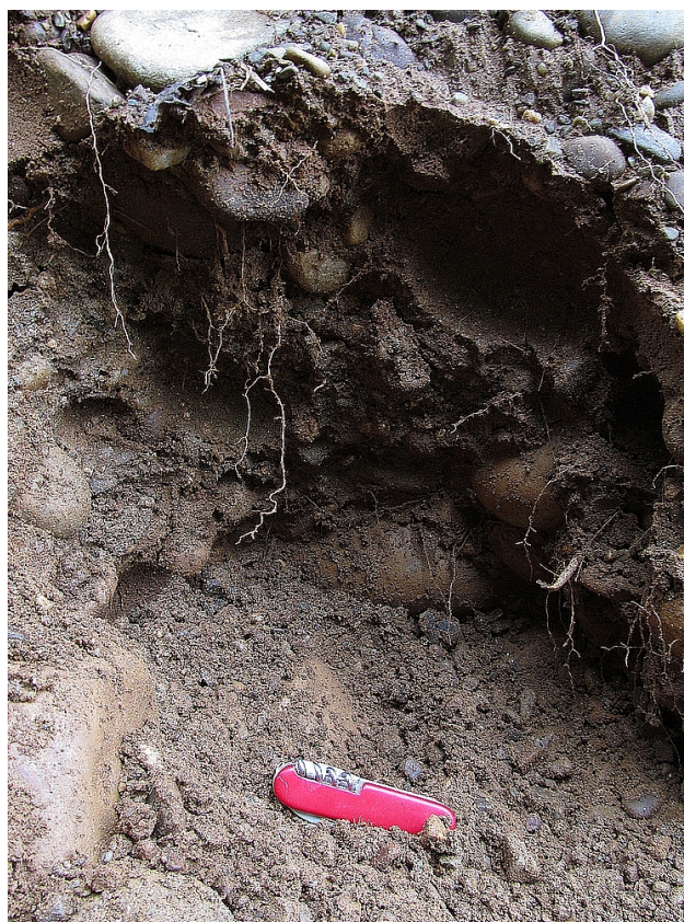
Figure A3. CDT3 - Sample from base of \sim 3.2 m thick fill of poorly sorted fluvial pebble and cobble conglomerate, suggesting it was deposited during a single event. Approximately 26 m above the modern channel. OSL dated at 9,760 \pm 1,040 years (Ray and Srivastava, 2010). 90 mm long penknife for scale.
