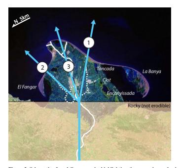
Figure 2. Schematic of modeling scenario, highlighting the succession and orientation of Ebro delta lobes, shown on top of the modern Ebro delta morphology (NASA Landsat image) and the inferred paleo channels (dotted lines, from Maldonado, 1975). In the model, the straight reference coastline is assumed to be non-erodible. Names refer to the spits and the lagoons on the Ebro delta. Numbers refer to the (1) Riet Vell, (2) Sol de Riu, and the (3) Mitjorn-Buda lobes.
