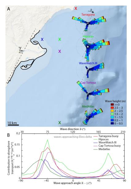
Figure 3: (A) Comparison of the five different wave roses and their location on a map from NOAA (2015). See table 1 for an overview of the sources. (B) Angular distribution of alongshore sediment transport potential for the five different sources.
