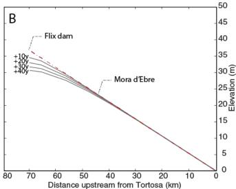
Figure 6. (A) A close-up of the Ebro drainage basin close to the delta (data from Google Earth, 2015). (B) Modeled response of the Ebro River downstream of the lowermost modern dam, the Flix dam. The bed degradation measurements from Vericat and Batalla (2006), are taken 25 km downstream of the Flix Dam, in Mora d'Ebre.
