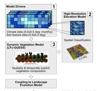
**Figure 2.** Schematic procedure of simulations. Coarse resolution model driving data (1) is disaggregated using a high-resolution elevation model and topographic landform classification (2) and the ecosystem model LPJ-GUESS then simulates vegetation state and dynamics using the landform classification to simulated topographic-adjusted patch composition (3). Vegetation cover and surface runoff results can then be passed on to a coupled landscape evolution (LE) model (not
