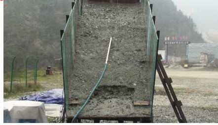
(c) Fine particles disappear and coarse particles are exposed
