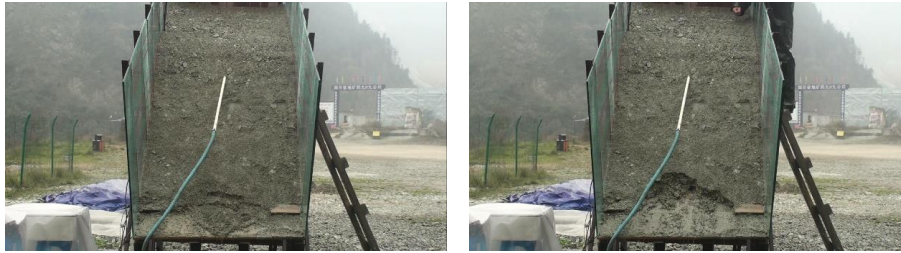
(a) Shearing opening appears at the slope foot
