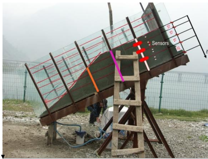
(a) Artificial flume model (the position of sampling: red line-1#, pink line-2#, white line-3#). (b) Grain composition of gravel soil.
