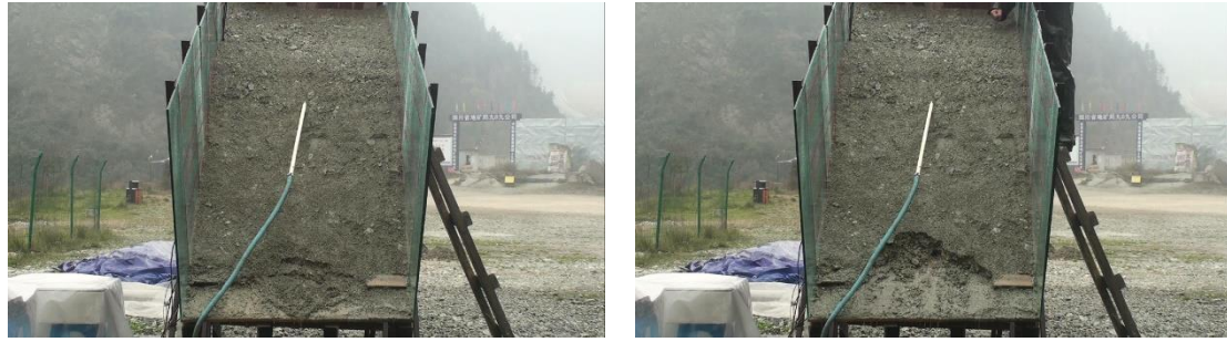
(a) Shearing opening appears at the slope foot
