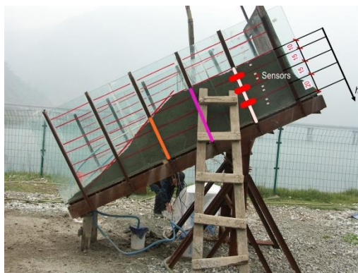
128 (a) Artificial flume model (the position of sampling: red line-1#, pink line-2#, white line-3#) (b) Grain composition of gravel soil
