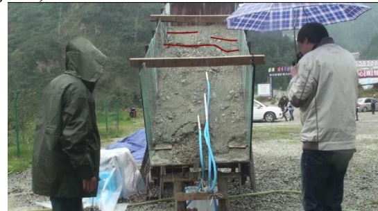
(b) Cracks develop on the slope top
