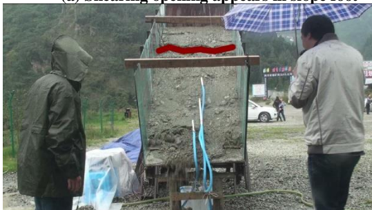
(c) Crack propagation
