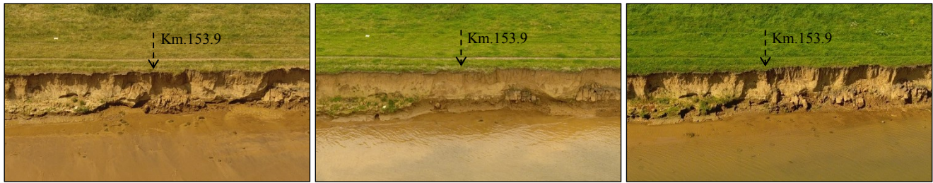
Figure 13: Zoomed-in UAV photos from track 1 at section 4, km. 153.9, showing diverse bank erosion stages: slump blocks at bank toe on June 21 (left), clean bank face after block removal on July 19 (centre), and undermining on August 23 (right).
