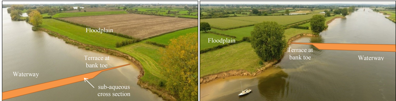
Figure 2: Restored bank in the Meuse River, upstream view of first 300 m (left) and downstream view of middle 500 m (right). Bank 20 erosion has caused a series of bays in the 1,200 meter restored reach. Note eroded bank sediment in suspension.
