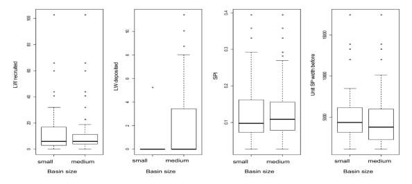
Figure: Boxplots of LW recruited  $(m^3/ha)$  and deposited volume  $(m^3/ha)$ , stream power index and unit stream power calculated with the estimated discharge and the initial channel width for small and medium watersheds following the classification by Seo and Nakamura (2009).
