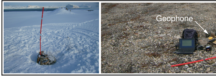
Figure A1. Photos of a station of the KBS array after deployment in April and a station of the BRA array during data retrieval in August (geophone uncovered).
