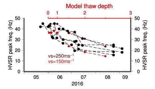
**Figure 5.** Comparison of observed HVSR peak frequencies for stations KBSA2, KBSA4, BRA2, BRA4, and BRA5 and modeled peak frequencies (taking into account anti-aliasing filter of seismic instrument). For the x-axis on top representing modeled thaw depth, we assume a square root dependency with time from beginning of June.
