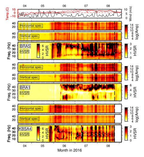
**Figure 3.** Same as Fig. 2 for three more stations. Grey dashed vertical line indicates change of color scale on July 10th. Color scale is clipped at high HVSRs (black) for KBSA4 and BRA5 to enhance visibility of the weak gliding peak at days of low wind speed. The scale used before July 10th is provided to the left.
