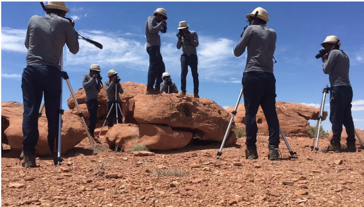
25 Figure 8. Multi-exposure image showing the different spatial positions from where images were acquired. First images were acquired from a distance of ~2 m then close-up images were taken from a distance of <~1 m. DEM and orthophoto of the imaged boulder is shown in Figure 10 g and h.
