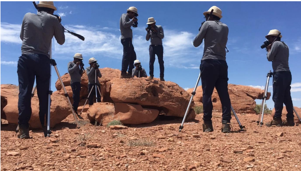
25 Figure 8. Multi-exposure image showing the different spatial positions from where images were acquired. First images were acquired from a distance of \sim 2 m then close-up images were taken from a distance of < 1 m. DEM and orthophoto of the imaged boulder is shown in Figure 10 g and h.
