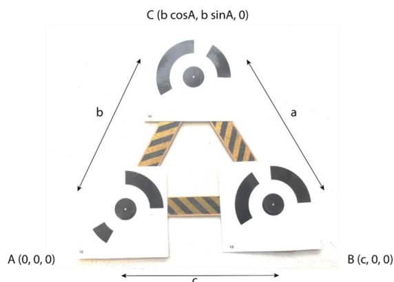
Figure 2. Triangle coded control target. Each vertex of this triangle is a GCP.
